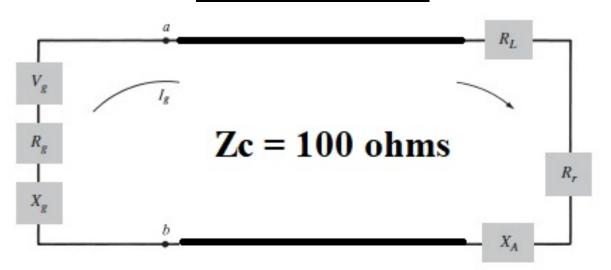
$$V_{g} = 10V, R_{g} = 50\Omega, X_{g} = 0$$
