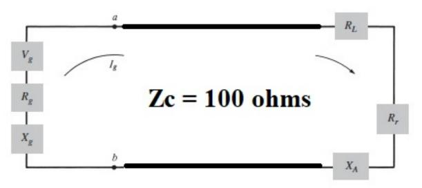
$$P_{r} = \frac{1}{2} \left| I_{g} \right|^{2} R_{r} = \frac{1}{2} \frac{\left| V_{g} \right|^{2} R_{r}}{\left( R_{g} + R_{in} \right)^{2} + X_{in}^{2}} = \frac{1}{2} \frac{10^{2} \cdot 48}{\left( 50 + 100 \right)^{2} + 100^{2}} = \frac{24}{15^{2} + 10^{2}} = \frac{24}{225 + 100} = \frac{24}{325} = 0.0738W$$
