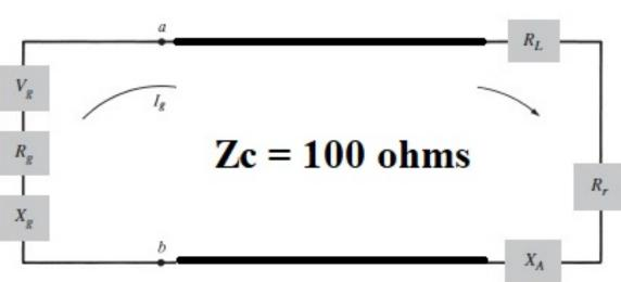
An antenna with a radiation resistance of 48 ohms, a loss resistance of 2 ohms, and a reactance of 50 ohms is connected to a generator with open-circuit of 10 V and internal impedance of 50 ohms via a  $\lambda/4$  – long transmission line with characteristic impedance of 100 ohms. Determine the power radiated by the antenna. Solution
